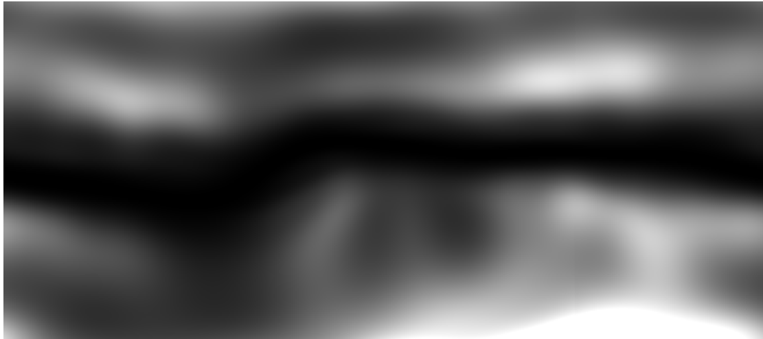
Figure 3: Map of the errors on the measurements of H-pol (6:00 AM, 45 degrees of incidence, looking across track). They range from 0 (black) to 0.00035 (white). Corresponding brightness temperatures errors may range from 0 to 0.11K for a 300K surface.
